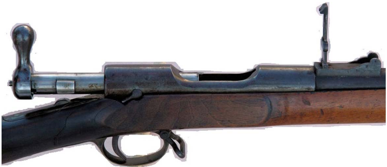
Fig. 7 – Brown-Merrill rifle with action open and rear sight leaf raised. Note that the hammer was cocked by the opening of the action. Note the locking lug in front of the bolt handle. Author's Collection, Photo Bill Chronister
