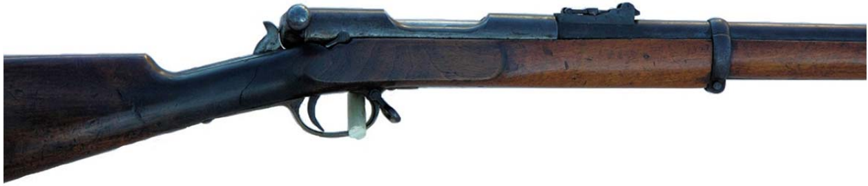
Fig. 5 - The Brown-Merrill action with bolt closed. Note the hammer behind the bolt, the small bolt locking latch in front of the bolt handle, the Pattern 1853 sight and the distinctive step in the stock by the barrel band. Note where the original lock plate was expertly replaced by wood. Author's Collection, Photo Bill Chronister
