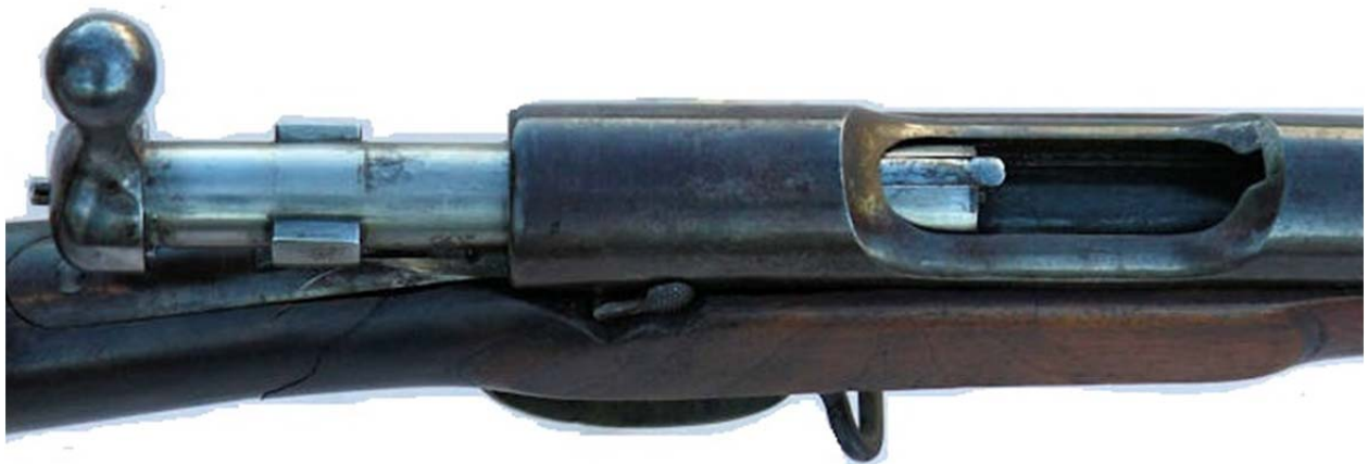
Fig. 8 – Top view of open action. Note the two locking lugs on the bolt, the extractor on the top of the bolt and the groove in the chamber that the extractor slides into. Author's Collection, Photo Bill Chronister
