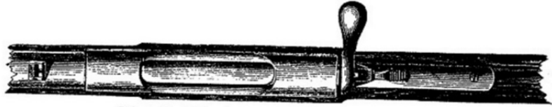
FIG. 6. Front View Lever and Hammer, in position to Fire.
